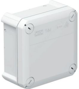
The junction boxes are made of a thermoplastic polypropylene polymer with closed side walls. This means that the required openings can be made wherever they are required. EDK plug-in seals or cable glands with locknuts can be inserted in these openings, to allow cable insertion. The junction boxes can be mounted on mounting plates in the openings on the floor using steel
